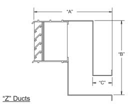
Fastened securely to vent 24 GA. galvanized steel standard. Use when space to be vented is below grade. Provide dimensions "A", "B", and "C".
